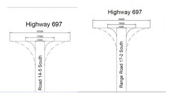
The intersections were found to be too narrow when compared to Alberta Transportation minimum standard. The intersections should be 30 metres wide plus the width of the road. These two roads are also narrow, compared to the Counties local roads.
